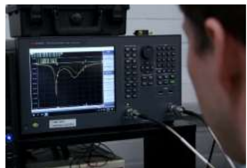
Figure 7. Antenna matching measurements using Vector Network Analyzer.
