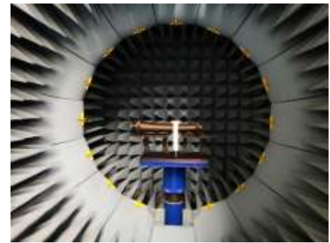
Figure 8. Antenna radiation property measurements using anechoic RF chamber.
