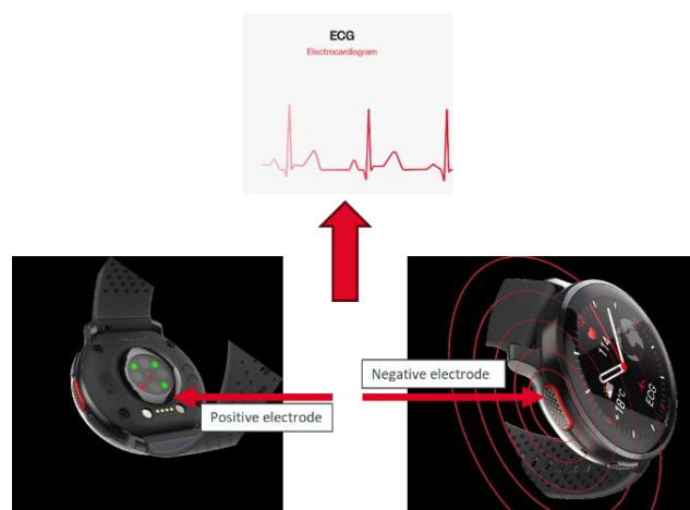
Figure 2. ECG-measurement principle of the wrist unit.
