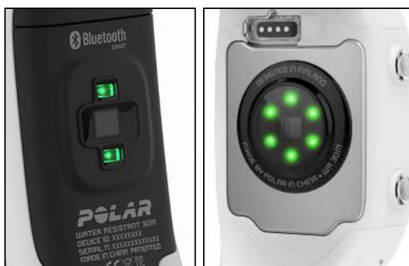
Figure 3. Optical measurement at the back of the wrist unit. Configuration a) two green LEDs as light emitters and one photodiode as the light detector between the LEDs; configuration b) six green LEDs around one photodiode.
