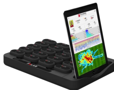
Figure 1. Polar Team Pro wearable sensors and a dock connected to an iPad for synchronization to the web service.
