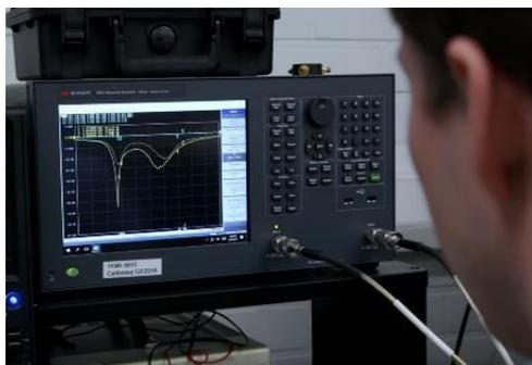
Figure 7. Antenna matching measurements using Vector Network Analyzer.
