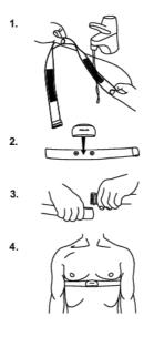
Detach the connector from the strap after every use, to maximize the transmitter battery lifetime. Sweat and moisture may keep the electrodes wet and the transmitter activated. This will reduce the transmitter battery life.
