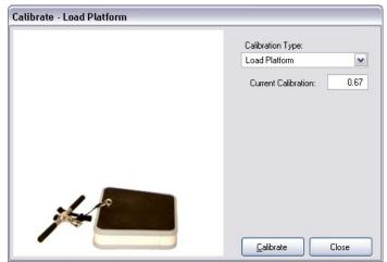
\*It is best to use a person that knows their exact weight and weighs between 68 and 86 kg to calibrate the scale, as weight plates are not always the exact weight as printed on them. Make sure the person has the same clothing on they were wearing when measuring and calibrating. The weight scale is accurate to within 0.2 kg.
